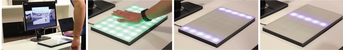
**Figure 3:** In the demonstration setup, an image viewer is controlled with gestures (image 1). When a gesture was recognized successfully, the device will light up in green (image 2). Forward clues are given by statically illuminating active regions (image 3) or animating swipe gestures with bars that move over the surface (image 4).
