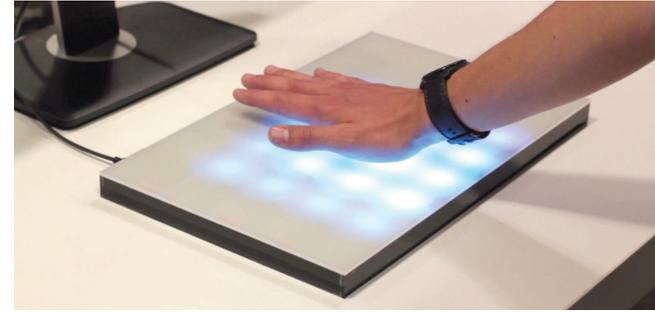
**Figure 1:** Rainbowfish is a capacitive gesture recognition system providing interactive feedback and feed-forward clues.
